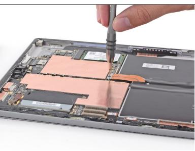
Remove the 3 mm T3 Torx screw securing the battery connector, and disconnect the battery connector.
