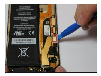
Disconnect the battery connection cable by using the plastic opening tool and applying light pressure upwards on the cable. To reassemble your device, follow these instructions in reverse order.
