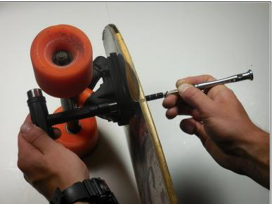
Use a Phillips/flat head screw driver, along with a skate tool or set of pliers, to loosen the nuts which fasten the trucks to the deck.
