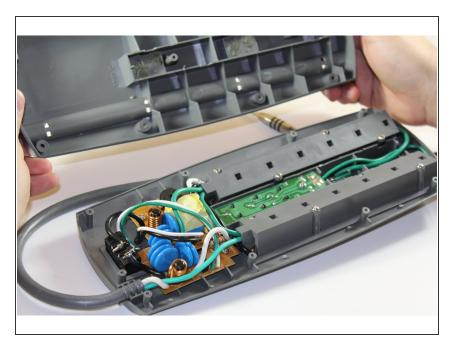
Remove the lower plate to expose the internal components.
