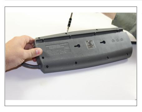
Remove the nine screws from the bottom plate using an IfixIt bit driver and the bit labeled PH1.
