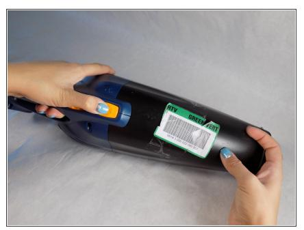
Pull the black nose off of the body of the vacuum, by pushing in the orange button closest to the nose.
