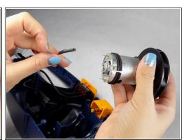
Pull your motor out, and remove the black and red cables from the motor by hand.
