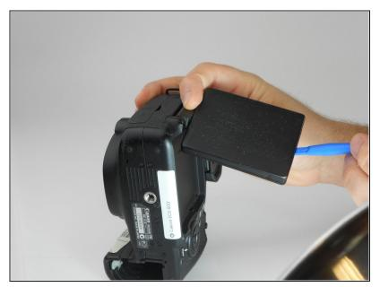
Using a plastic opening tool, carefully pry off the back cover of the LCD.
