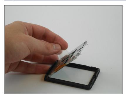
Finally, remove the LCD screen by grabbing the clear plastic tab and lifting it carefully.
