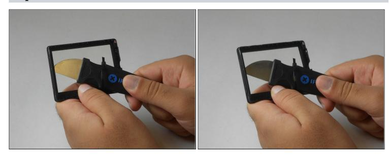
• Carefully slide the Jimmy through all corners of the plastic frame until it is detached from the plastic cover.
