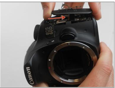
Using the plastic opening tool, carefully pry off the the side cover.
