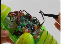
Use <u>tweezers</u> to remove all of the colored wire connectors from their sockets on the circuit board.
