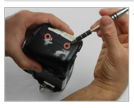
Remove two 4.8 mm Phillips #PH00 screws from the memory card side of camera using the PH00 screwdriver.
