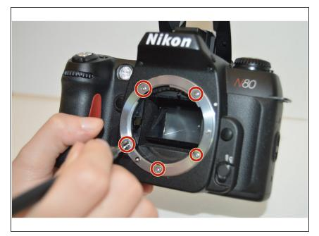
Use a PH00 Phillips screwdriver to remove the five 4.8mm screws on the silver lens mount.
