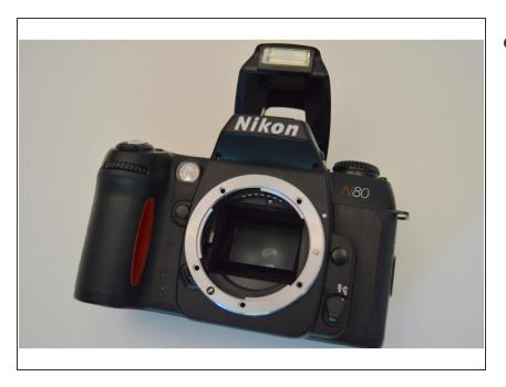
Remove the old lens mount and place the new one on.
