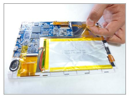
Remove the yellow tape from the sides of the battery, and the surrounding components.
