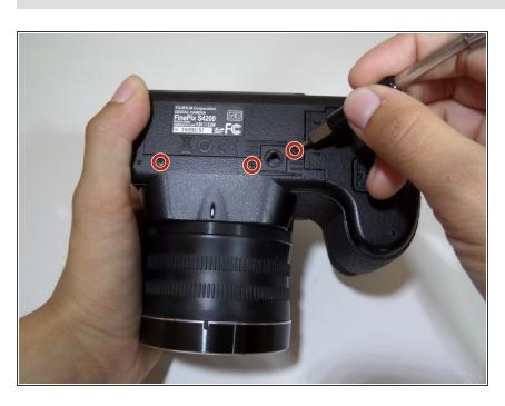
Remove the three 4 mm screws from the bottom of the camera with a Phillips #000 screwdriver.
