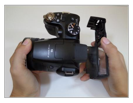
Use force to pull apart the back casing from the camera.
