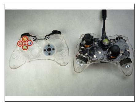
Remove the rubber button covers from the A, B, X, and Y buttons.
