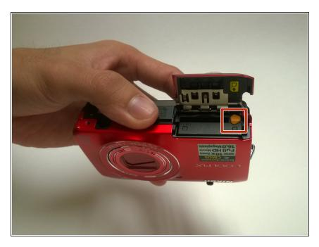
Rotate the orange battery clip in the camera to release the battery.
