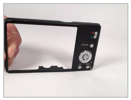
Using the plastic prying tool, remove the cover of the camera that is on the same side as your LCD screen. This cover should come off relatively easily, and will expose the motherboard that the screen is connected to.
