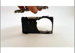
• After the front panel is removed, the buttons are connected by a simple string of clips. To remove the buttons, find the clip on the back and the two on the front that are connecting the buttons to the shell of the camera. Remove these clips and pull the buttons up from the back at an angle towards the front to remove them.
