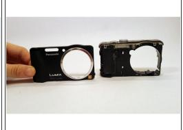
Once the motherboard has been removed, flip the camera over and remove the front panel.
