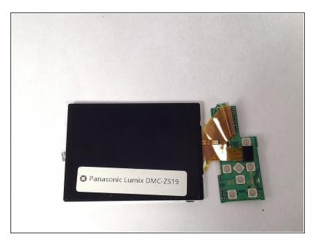
Using your hand, follow the two data-strips that connect the LCD screen to the motherboard and unclip them. Once the data-strips are unclipped, remove them from the motherboard and the screen will be free.
