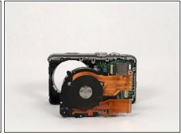
Once the plastic riser is removed, it is time to remove the lens. To do this, simply follow the data strips (2) that connect the lens to the main motherboard and unclip them by turning the black bar into a position that is perpendicular to the motherboard. Once these clips are open, the data strips and the lens should simply slide out.
