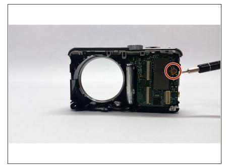
After the lens has been removed, there is only one screw that holds the main motherboard in place.
