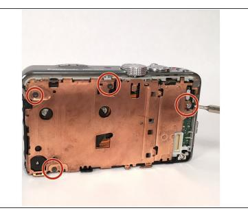
• After the screen has been removed, the main motherboard is directly underneath it. There is a bronze, metal separation piece that separates the main motherboard from the one connected to the lens. This metal piece is held in with 3 screws. Remove these 3 screws and the metal piece will be free.
