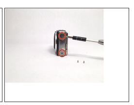
Locate the pair (2) of screws on each side of the camera and remove them. Then locate the pair
