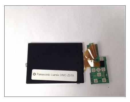
Disconnect the motherboard that the LCD screen is connected to from the main motherboard.
