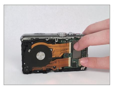
Once the bronze metal plate is removed, the main motherboard will be exposed. There is a plastic riser (it looks like a lowercase "b" on the right side of the camera) that separates the metal plate from the motherboard. Remove this plastic riser.
