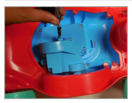
Put three 1.2mm screws for the motor back into place.
