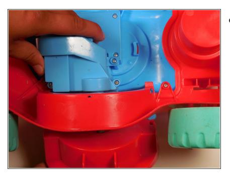
Insert the Bubble sprocket onto the motor.
