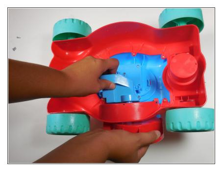
Remove the Bubble Sprocket from the motor.
