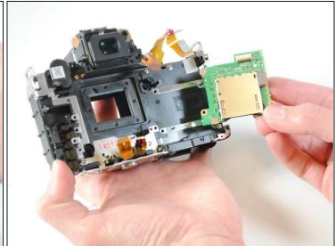
• Using your fingers, remove the SD card reader from the back of the device.
