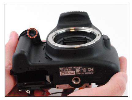
Remove the black 5 mm Phillips #000 screw, located under the grip.
