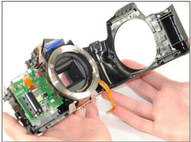
• Remove the front panel of the camera.
