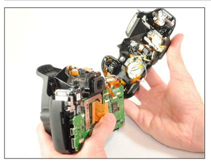
• Remove the top panel of the device.
