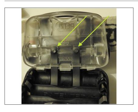
Remove the batteries and lift the two straps with a flat screwdriver. Pull the straps out.
