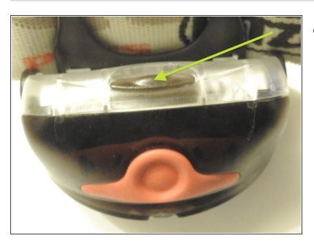
Push the catch on the top to open the battery compartment
