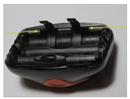
This is the most crucial part. Do NOT try to release the latches at the front. Insert a small screwdriver at the positions indicated in the back near the "belt hinges" to flex the rear part of the case back and free the latches of the inner part.
