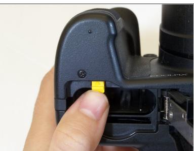
Once the battery cover is open, push the solid yellow tab in the direction of the arrow. This will then eject the battery out of the camera.
