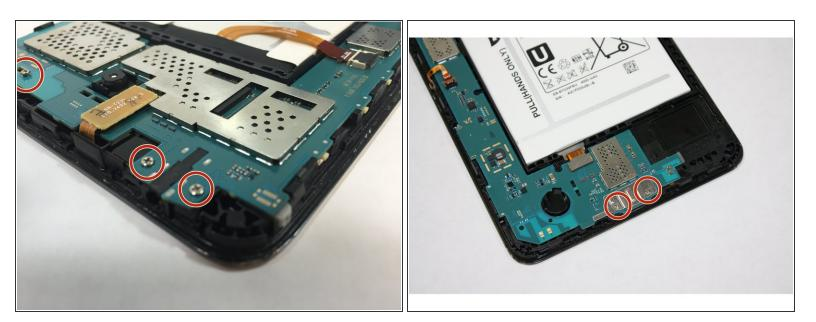
Use the Phillips 000 screwdriver to remove the remaining five 1.2 mm screws.
