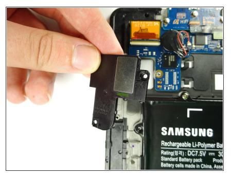
• Lift and remove the speaker from the device once the screws have been removed.
