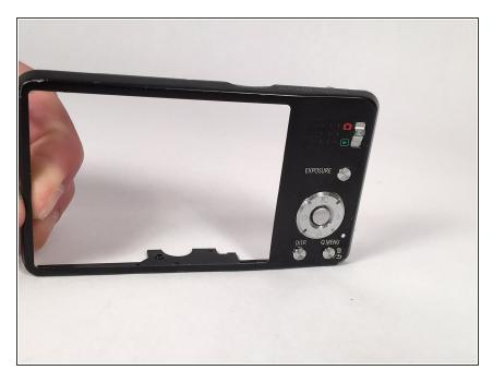
Gently remove the loosened panel from the LCD screen.
