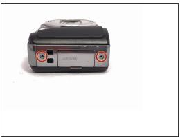
Start by removing the screws located on the left and right hand side panels of the camera (two sets of pairs of screws). Next remove the pair of screws on the bottom of the camera. (6 in total)
