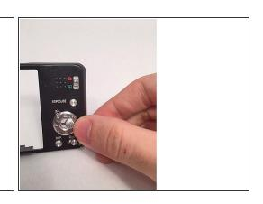
Carefully use a finger to pop out the Menu/Set button from the panel by pushing on it.
