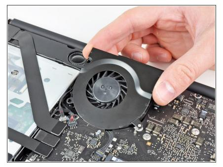
• Lift the fan out of its recess in the logic board, minding its cable that may get caught.
