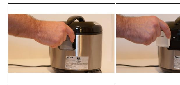
• The first step is removing the condensation catcher in order to reach the control panel. We do this by pinching the condensation catcher as shown, on both sides and pull the condensation catcher away from the cooker.
