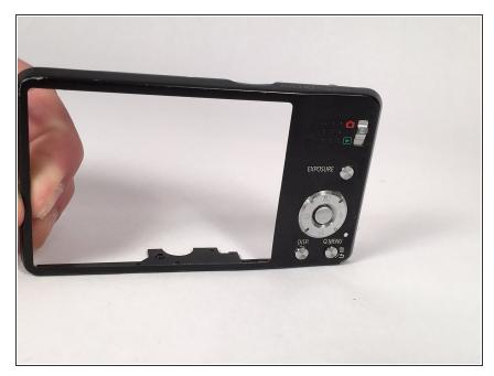
Using the plastic prying tool, remove the cover of the camera that is on the same side as your LCD screen.
