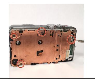
After the screen has been removed, the main motherboard is directly underneath it. There is a
