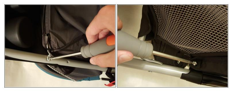
• Using a Phillips #1 screwdriver, remove the twelve 12 mm screws and set them aside.
