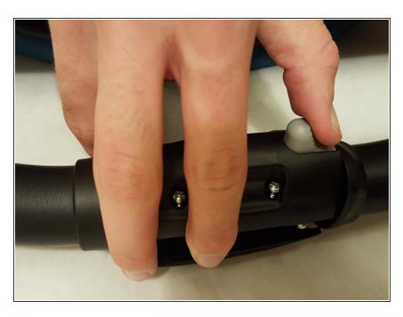
Push the switch in to allow the handle cover to come free.
