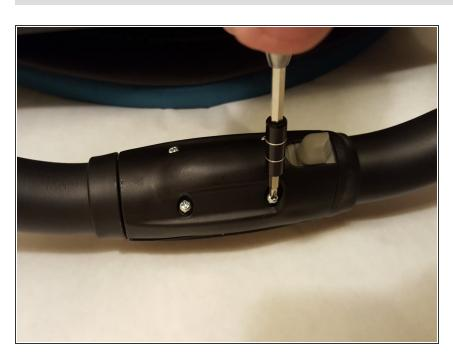
Using a Phillips #1 screwdriver, remove the four 22 mm screws and set them aside.
