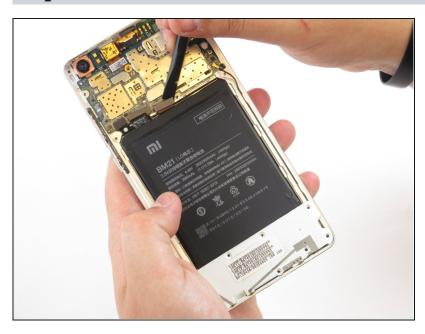
Use a spudger to pry upwards and detach the three ribbons that are connected to the motherboard.
