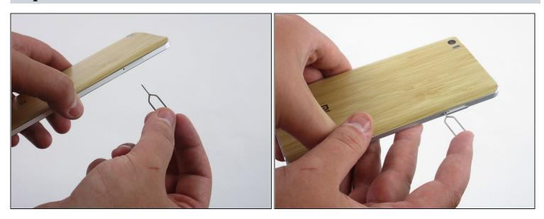
• Use the Dual SIM SD card removal tool (or use a paper clip) and insert it into the slot hole until the tray pops out.
