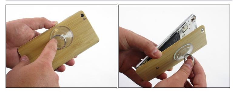
• Use your suction cup to grip the back of the phone. Once the suction cup is secure, pull back with moderate force and the back plate should snap free.
