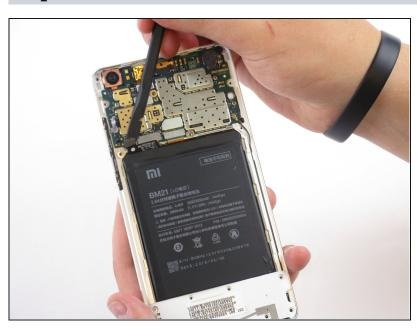
Use a nylon spudger to pry upwards to detach the ribbon that's connecting the battery to the motherboard.
