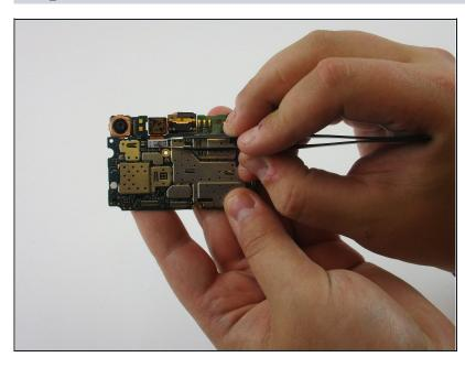
The front camera is attached to the motherboard by a ribbon, use tweezers to detach it from the motherboard.
