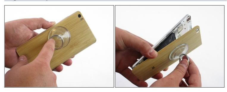
• Use your suction cup to grip the back of the phone. Once the suction cup is secure, pull back with moderate force and the back plate should snap free.
