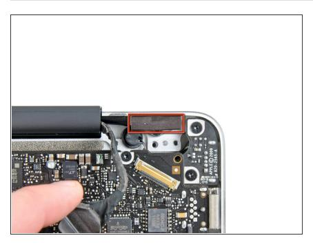
Remove the piece of foam tape covering the display screws near the MagSafe DC-In board.
