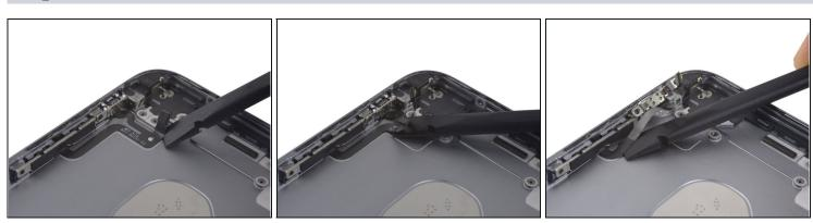
• Use the flat end of a spudger to peel up the volume control flex cable.
