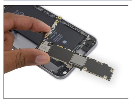
• Remove the logic board.
