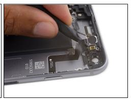
• Insert the tip of a spudger underneath the microphone portion of the flex cable and gently pry it off of the rear case.
