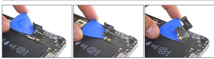
• Insert an opening pick under the Lightning connector flex cable and slowly slice through the adhesive holding the cable to the rear case.
