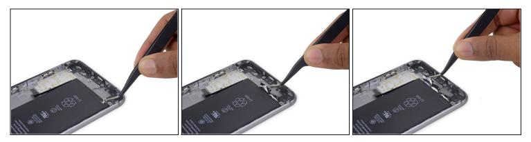
• Use a pair of tweezers to peel back the tips of the three battery adhesive strips along the bottom edge of the battery.
