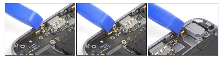
• Use an opening pick to pry the left microphone off the edge of the rear case.
