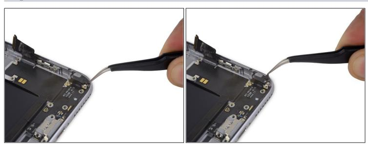
Peel back the tape over the screw securing the Lightning connector flex cable to the lip of the phone.
