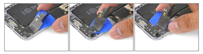
• Continue sliding the opening pick underneath the flex cable.
