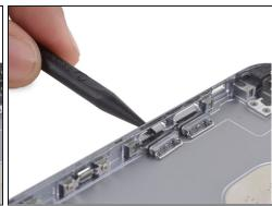
• Use the pointed tip of a spudger to nudge the volume control button covers out of their slots in the rear case.
