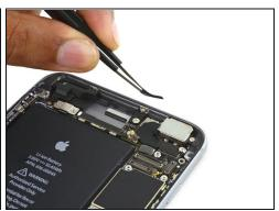
• Peel up any tape covering the iSight camera bracket screws.
