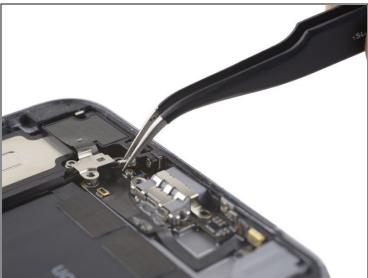
• Use a pair of tweezers to disconnect the Wi-Fi diversity antenna cable from the Lightning connector flex cable.
