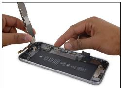
• Tip the logic board up to a vertical position to expose the single antenna connector on the underside, near the top edge of the board.
