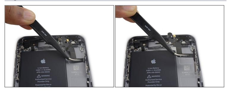
• Remove the power button flex cable.
