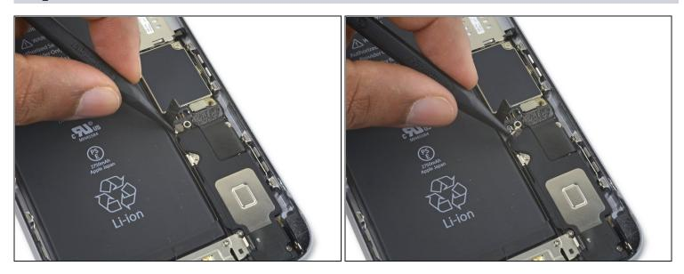
• Disconnect the antenna cable by prying it up from the logic board.
