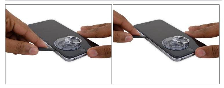
• Slide the tip of the spudger up the left side of the phone, between the front panel and the rear case.
