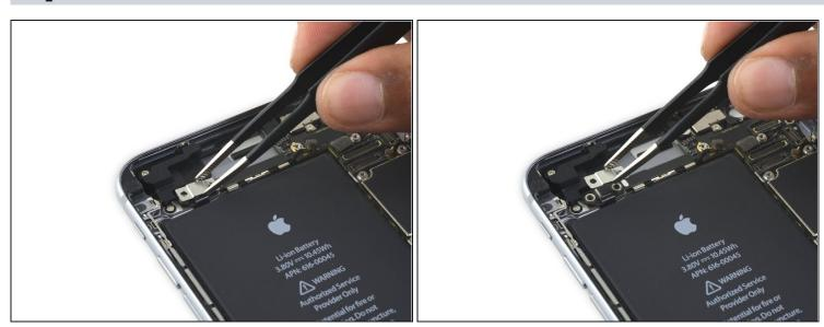
• Remove the audio control cable bracket.
