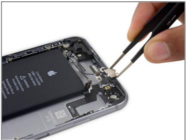
• Remove the flash/microphone bracket.
