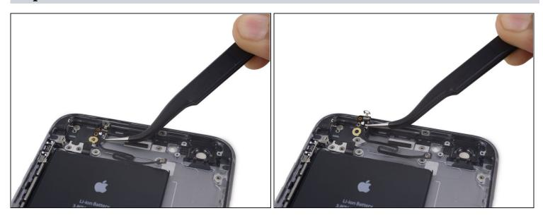
• Remove the Wi-Fi/Bluetooth antenna.
