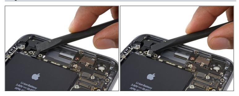
• Disconnect the audio control cable by prying its connector straight up from its socket on the logic board.
