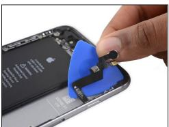
• Slide an opening pick underneath the power button flex cable to pry the cable off the rear case.
