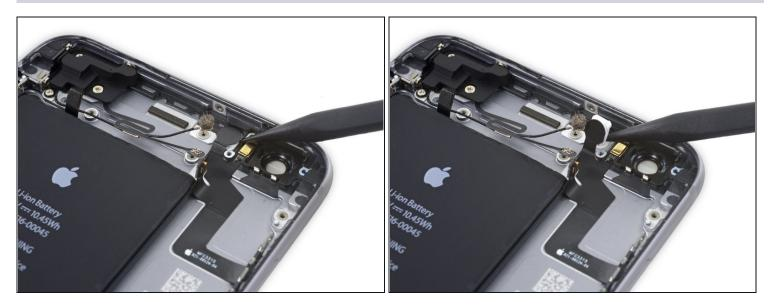
• Use the pointed end of a spudger to lift the flash out of its housing in the rear case.
