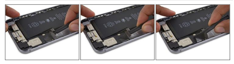
• Use the flat end of a spudger to peel the Lightning connector flex cable off the speaker.
