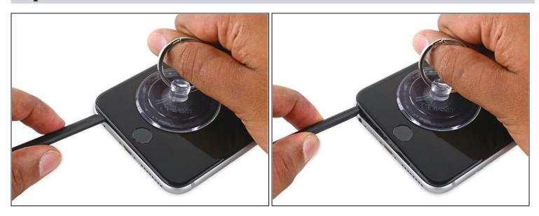
• Twist the spudger to widen the gap between the front panel and the rear case.
