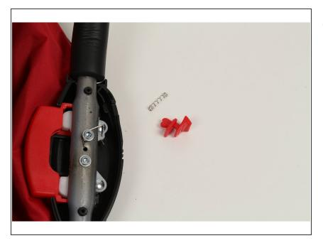
If the spring does not come out when you remove the "Free-Stand" button, lift the spring out of the case so it can be fixed or replaced.
