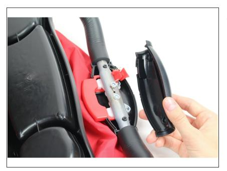
Remove the back cover of the case by lifting it straight up.
