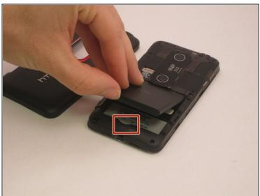
• Remove the battery with your hands, lifting at the marked area.
