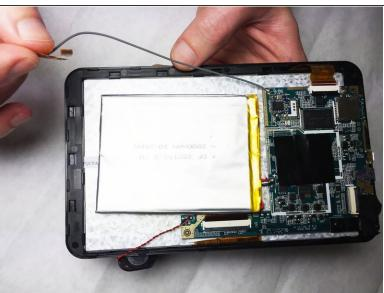
Detach the end of the Wi-Fi antenna from the tape on the edge of the shell.
