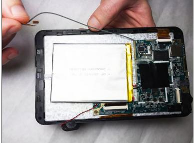
Detach the end of the Wi-Fi antenna from the tape on the edge of the shell.
