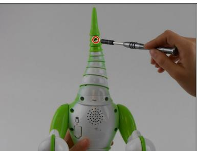
Remove the 9.4 mm Phillips #0 screw from the bottom of the tail of Zoomer Dino Boomer.
