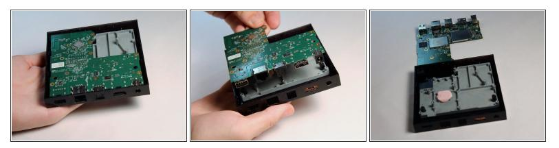
Place your finger on the short edge of the motherboard and lift it to separate it from the plastic case.
