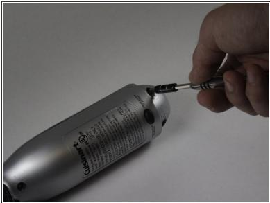
Remove three 13.3 mm Phillips PH#2 screws.
