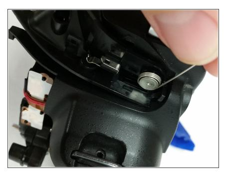
Remove the spring by sliding it off, then replace it with a new one.
