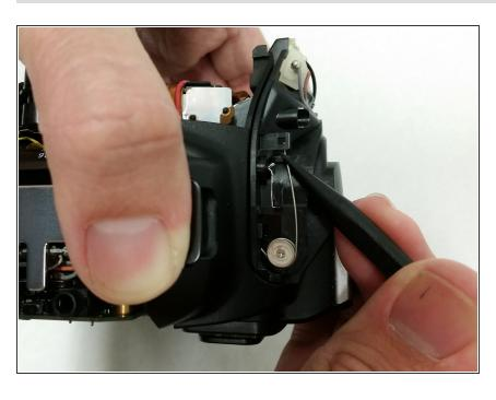
Lift the flash arm spring using the plastic spudger and unhinge the spring to remove it.
