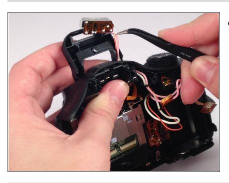
Use a soldering tool to remove the three wires connecting the flash to the camera.
