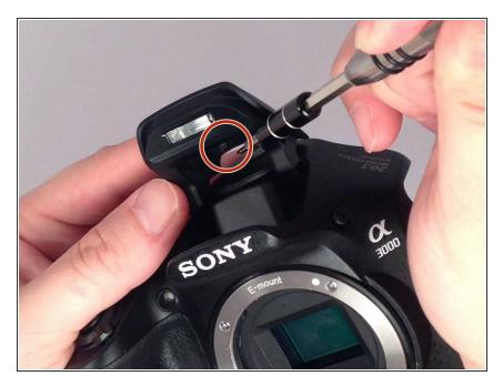
Remove the single screw from the bottom of the flash device.
