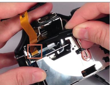
Gently but forcefully lift up on the parallel cable connecting the two halves of the camera.
