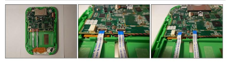
Disconnect the three wires that will be visible on top of the motherboard. The wires need to be disconnected by pulling them up vertically.
