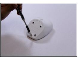
Remove the 9mm screw from the battery cover of the nursery unit using a Phillips #1 tip screwdriver.
