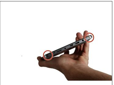
• Remove the (4) 3.5mm screws using a phillips #000 screwdriver.
