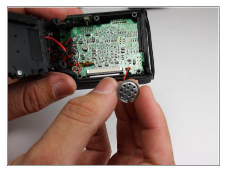
Remove the wires connecting the speaker to the motherboard from the motherboard, and <u>solder</u> the wires connecting the new speaker to the motherboard in the same locations as the wires that were removed.
