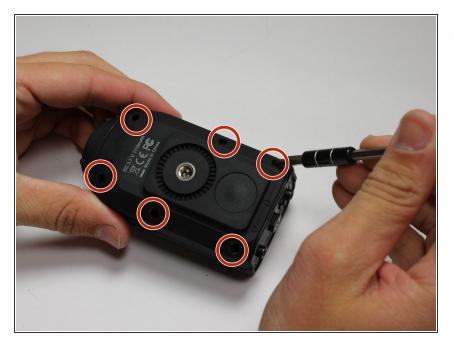
Remove six 8mm long Philips head screws with the J0 Philips head from the outer case.
