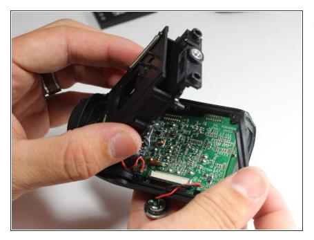
• Remove the battery housing from the camera body.
