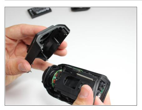
• Remove the back case from the camera body.
