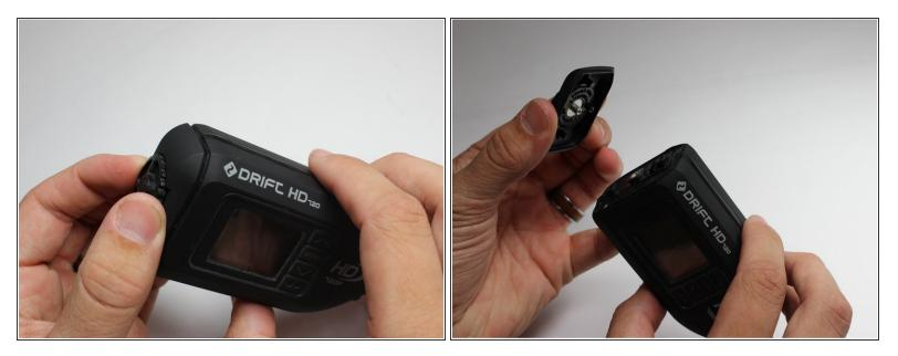
• Unscrew the back plate counterclockwise until it comes off.
