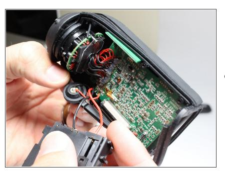
Remove the microphone first from the rubber housing it is located in, after which you will disconnect the wires connecting the microphone to the motherboard from where they are attached on the motherboard. You will then solder the new speakers wires in the same locations on the motherboard as the wires you just removed.
