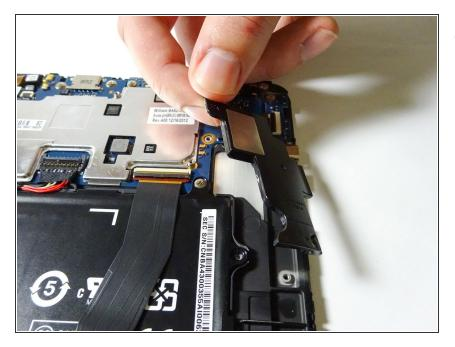
• Once the screws have been removed, lift and remove the speaker from the device.
