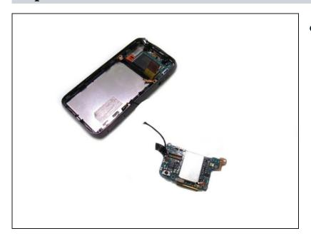
• Carefully remove the circuit board from the device.
